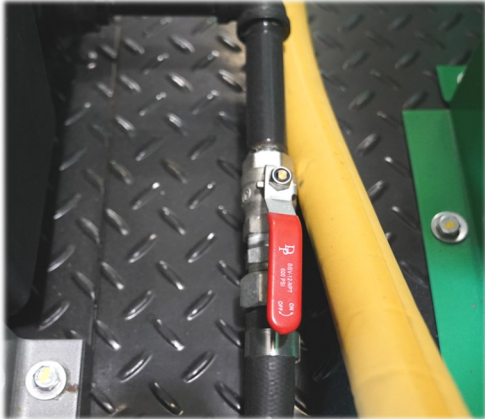
Figure 6. Valve is pictured in the open position
