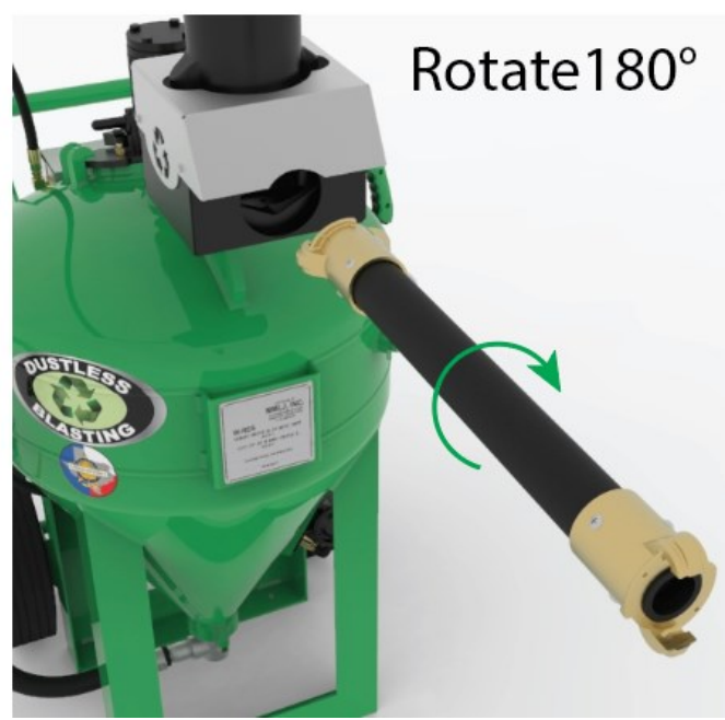
Figure 12. Rotating the pinch hose
